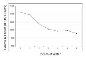
Figure 4: Gamma ray attenuation in water.
