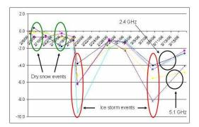
Figure 5: Susceptibility of microwave radiation to winter storm events having significant water content (R). Horizontal scale is in days, vertical scale is in relative attenuation in dB.
