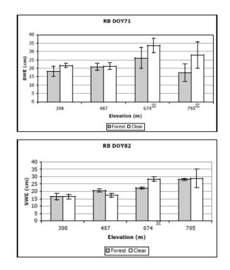
Figure 7: SWE differences at forested and cleared sites, Ranch Brook (RB) watershed, Vermont. Mean and standard deviations are based on 3-5 samples per site collected on March 12 (DOY 71) at peak accumulation and March 23 (DOY 82), after snowmelt commenced in 2007. Asterisks represent significant differences in mean SWE at  $\alpha = 0.05$ .
