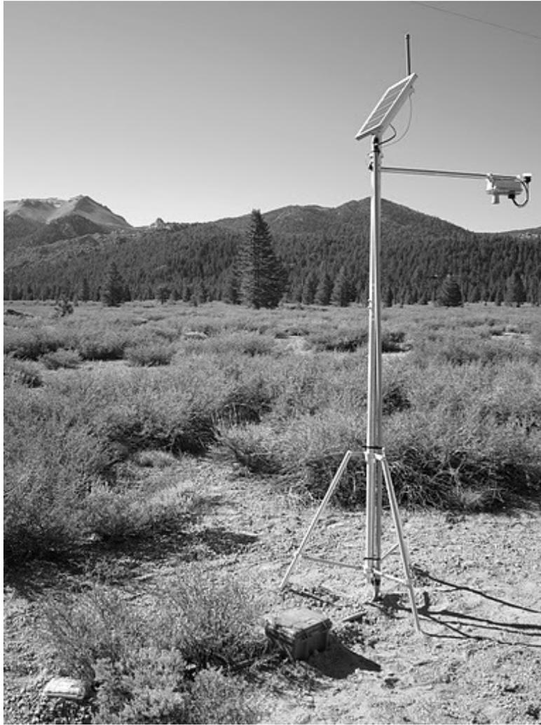
Figure 4: Snowcloud WSN sensor tower. A complete sensor stand with solar-recharged battery power, wireless mesh communication, and multiple sensor modalities. October 2011, Mammoth Mountain, CA.
