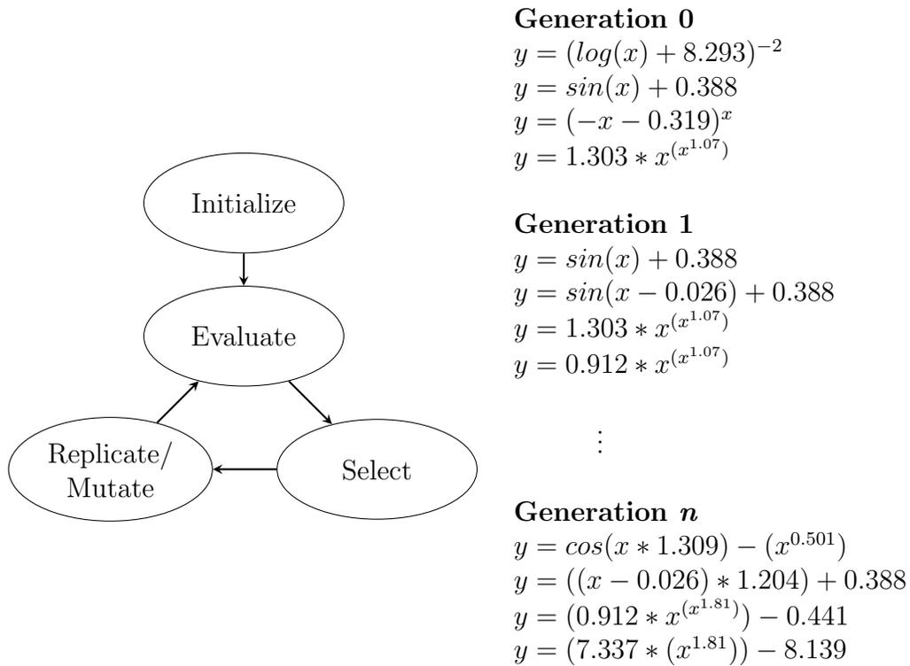
Figure 6: Genetic programming algorithm. The figure on the left demonstrates the iterative process through which GP modifies a population of solutions over time. On the right, a population of four models evolves as each iteration of the GP cycle produces a new generation.
