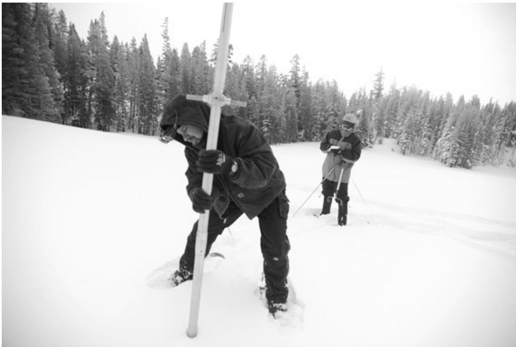
Figure 5: Manual snow survey. Gene Gutenberg drops a sampling tube into the snow along California's Highway 88 at Carson Pass. Kelly Cross records measurements (Kellum, 2014).
