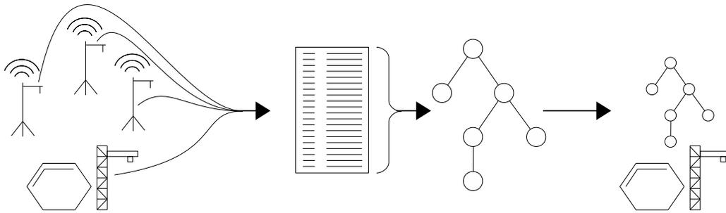
Figure 1: Using machine learning to model snowpack. First, the Snowcloud wireless sensor network is deployed in an area near a snow pillow to collect distributed ground truth data. Next, data generated by Snowcloud, by the pillow, and potentially other sources, is used by machine learning to generate a model of snowpack distribution. Finally, after Snowcloud has been removed, the model is used to estimate snow levels in the area where Snowcloud had been deployed.
